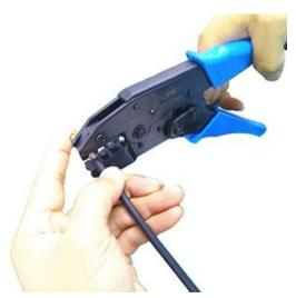
4. Insert the cable with copper conductor into the connector body:
